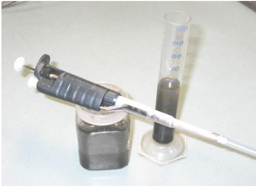
Fig. 4a: Gilson autopipette used to extract 1 ml from agitated trap sample
